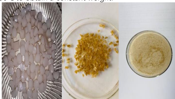
Fig 1: Photo of (a) preparing and cutting (b) drying (c) grinding of hydrogel Nano composite
