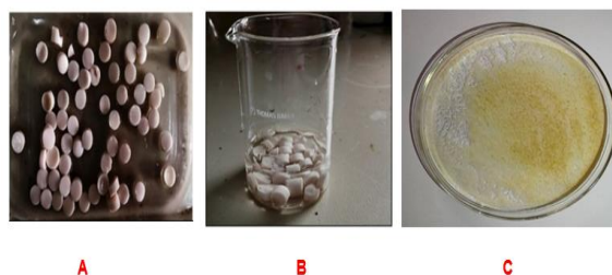
Fig 1: Photo of (A)preparing and cutting(B)washing (C)drying and grinding of hydrogel Nano composite.
