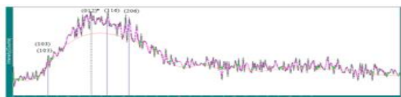
Fig.(3):The XRD spectrum of iron oxide nanofilm annealed at 300°C for 2 hours
