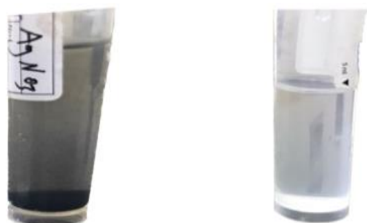
Figure 1: Color change of the silver nanoparticles solution
