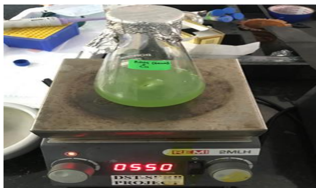
Figure 3: showing the process of magnetic (auto heated) stirring of Silver nanoparticle extract solution.
