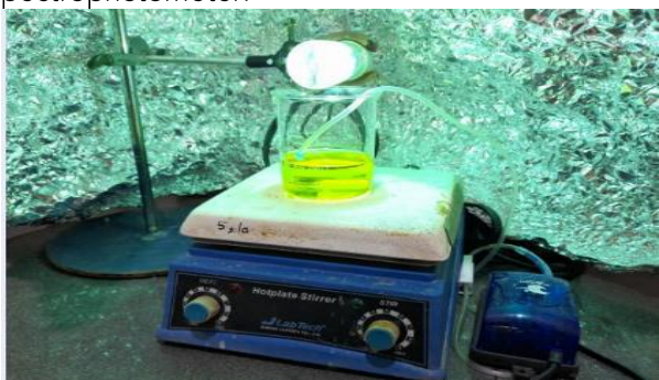
Fig.2: The photocatalytic cell's main components in the photocatalytic degradation of Orange G dye.
